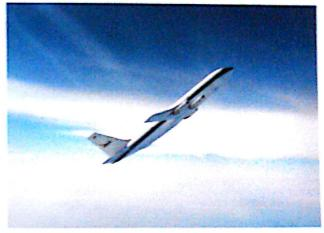
environment simulating zero gravity is created within the plane. This effect can cause some nausea in the participants, giving rise to the name "Vomit Comet", the plane used by NASA for zero-G parabolic training flights. Currently there is a private company that will sell you a zero-G ride, though it is a bit expensive.
